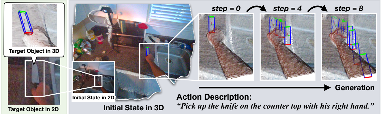
Figure 1. 6DoF object manipulation trajectory. This task aims to generate a sequence of 6DoF object poses from an action description and an initial state comprising the visual input and the object’s initial pose.
