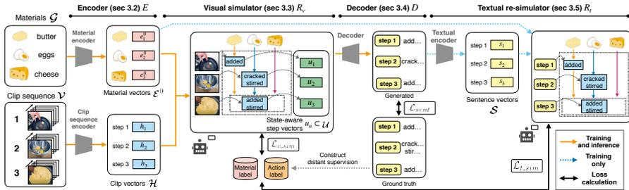
**Fig. 2** An overview of the proposed method. To track material states in a clip sequence, we incorporate the visual simulator  $R_v$  into the transformer-based encoder-decoder architecture ( $E$  and  $D$ ). In addition, based on our intuition that the state transition of materials is traceable from the generated procedural texts, we attach the textual re-simulator  $R_t$  to the model.
