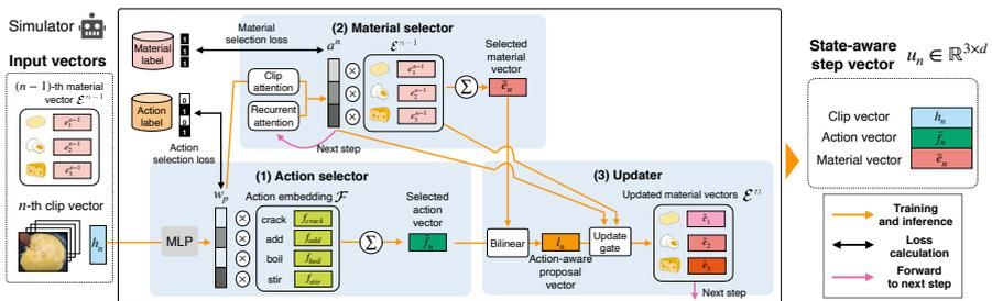
**Fig. 3** An overview of the (visual) simulator. The simulator recurrently reasons the state transition of the materials at each step. Specifically, it predicts executed actions and involved materials in (1) the action and (2) material selector and then updates the state of materials in (3) the updater. The updated materials are forwarded to the next step. The textual re-simulator has the same modules.
